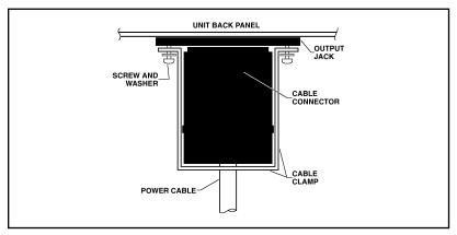
Figure 4.1: Output Cable Clamp Installation
